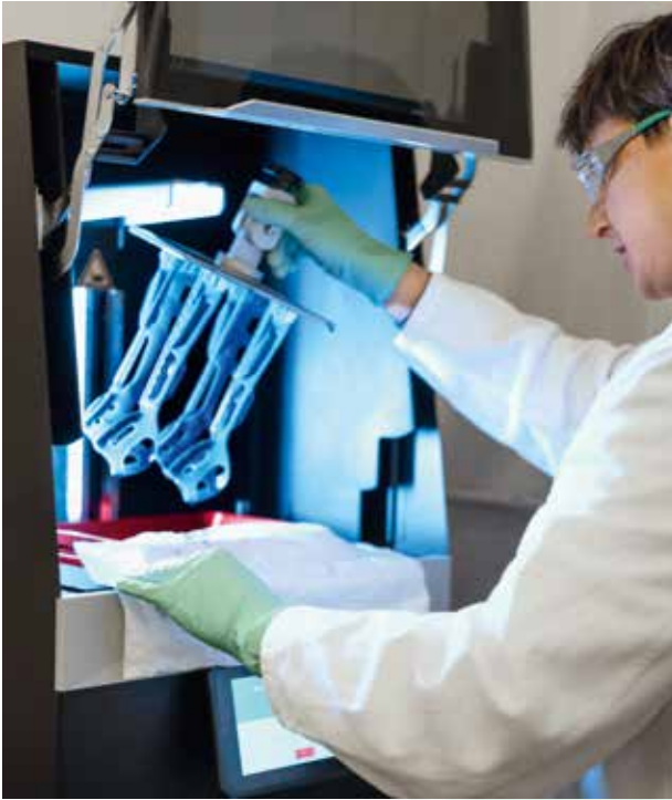
Off to the sunbed: Cubic Ink® has purchased 15 3D printers to expedite material testing processes. Following the printing phase, the initial step involves curing the printed materials.
