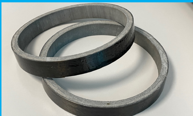
Filament winding for structural reinforcements.
