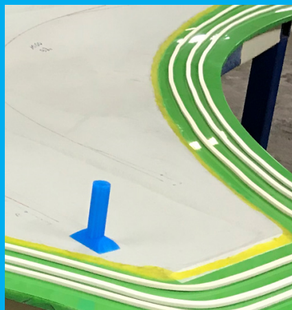
Vacuum bagging in silicone, for PE and EP systems.
