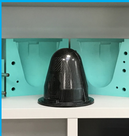
Aerospace Carbon Composite molded into EB 690 epoxy board mold.
