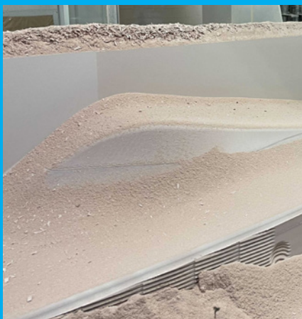
Master model production with medium density modelling paste, machine applied.
