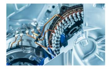
insulation system is a key parameter in achieving long machine life times. Therefore a successful combination of wire enamels, flexible insulation materials and impregnating as well as casting & potting resins is in demand.
