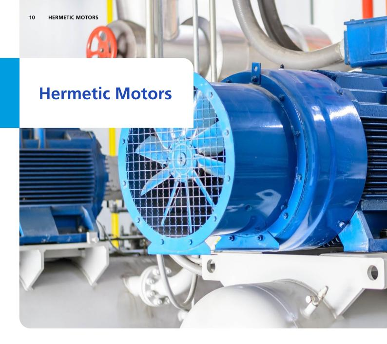
Hermetic motors are designed to operate in harsh chemical environments, and so demand a high level of protection against exposure to refrigeration-based gases, oils and contamination.
