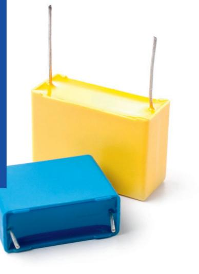
Film and foil capacitors are the most commonly used capacitors in the industry. Their essential differentiator is the dielectric used and its properties.
