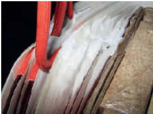
Intermediate insulation of transformer
